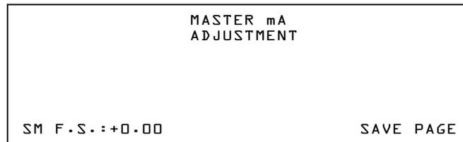
**4. Make a master adjustment of mA leading edge for Large focal spot.**
