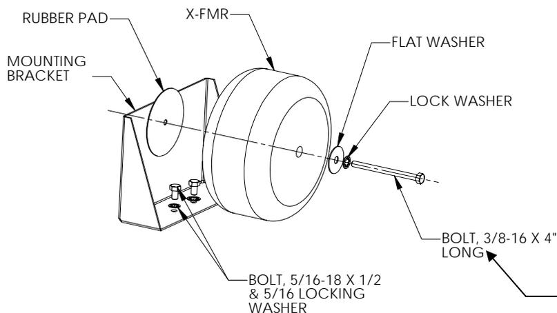
**WARNING: DO NOT CONNECT ANY WIRES TO THIS MOUNTING BOLT**
