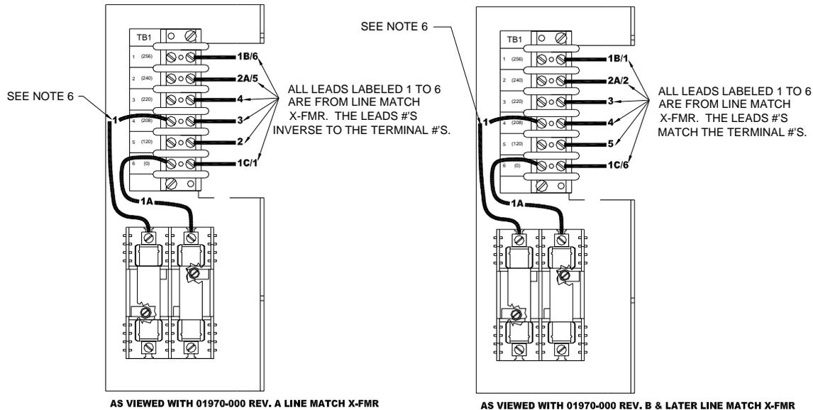
6. On the left side of TB1, locate the wire labeled “1”. This is the line voltage adjust wire. Move wire “1” to the TB1 tap which most closely matches the incoming line voltage (208 VAC or 220 VAC).
