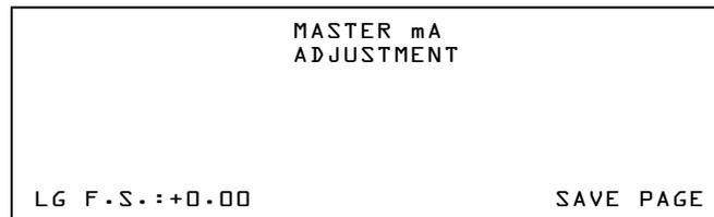
Using the same kVp and time, now select 300 mA and verify mA output. If adjustment of mA leading edge is needed at 300 mA, press the MASTER mA button, change the LG F.S. number and SAVE as before. Press the BACK button and repeat as needed to achieve the desired mA amplitude and mAs.
