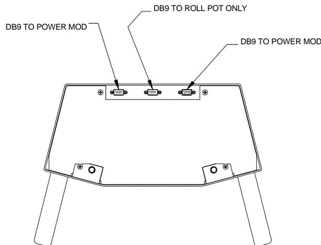
1. Remove the two ¼-20 cap head screws and washers located in the mounting holes at the bottom of the operator's console. Use this hardware to mount the operator console to the tube arm. Ensure hardware is tight.
