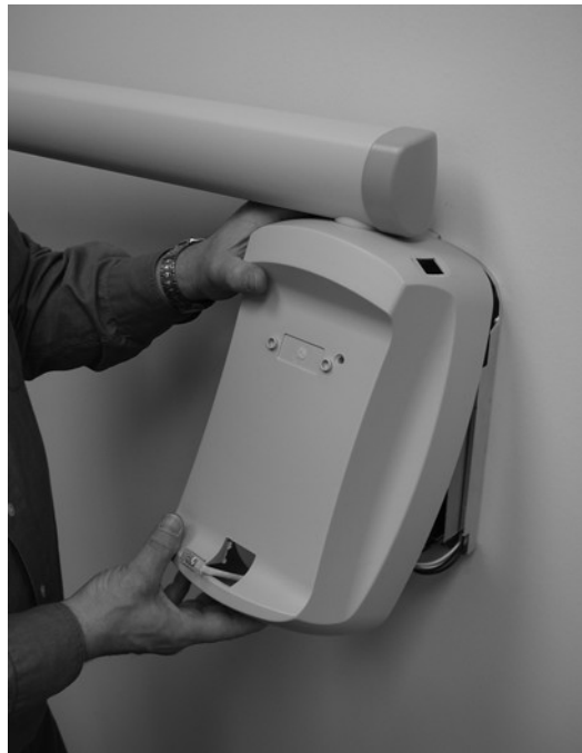
Figure 29 Placing the Cover on the Control Unit
