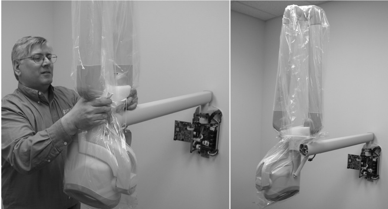
Figure 18 Installing the Articulating Arm and Tubehead Assembly
